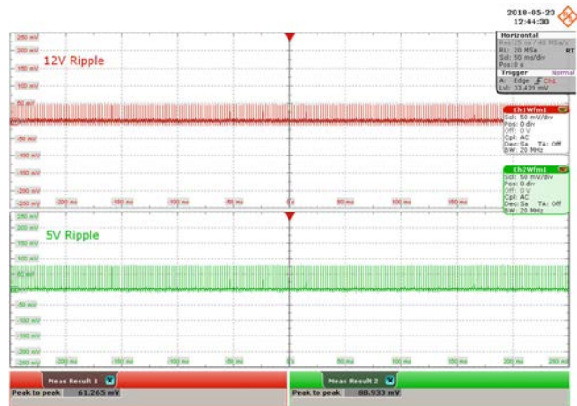
Figure 26 – 115 VAC Input. Vertical: 50 mV / div. Horizontal: 50 ms / div. 12 V Ripple: 61.265 mV PK-PK . 5 V Ripple: 88.933 mV PK-PK .
