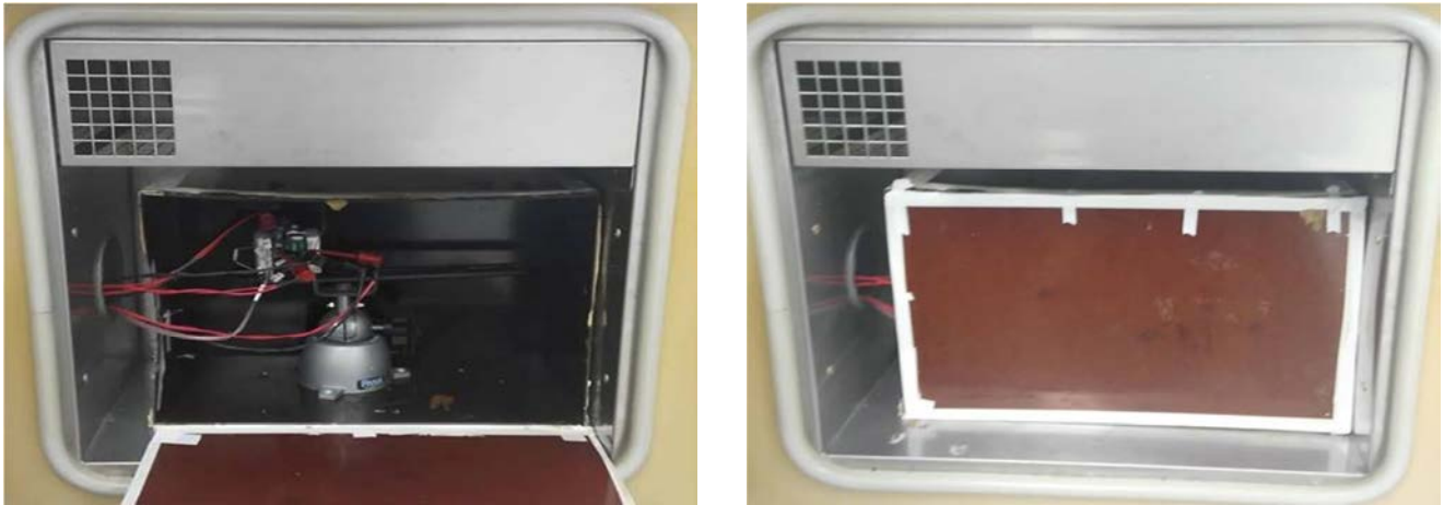
Figure 74 – Thermal Performance Set-up Using Thermal Chamber.
