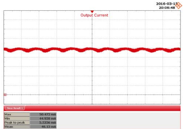
Figure 68 – 230 VAC, 50 Hz, 385 V LED Load. Upper: I_{OUT} , 10 mA / div., 10 ms / div.
