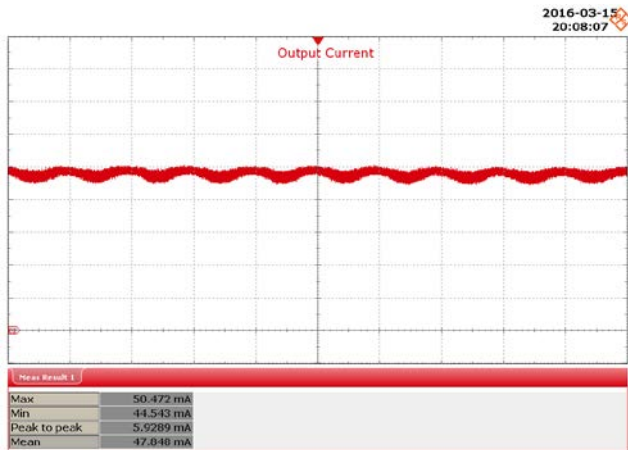
Figure 67 – 195 VAC, 50 Hz, 385 V LED Load. Upper: I_{OUT} , 10 mA / div., 20 ms / div.
