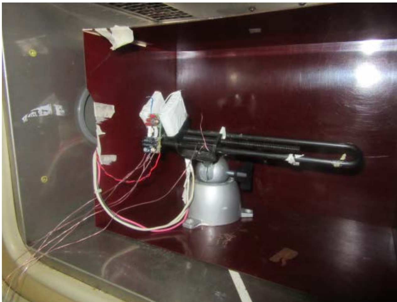
Figure 20 – Test Set-up Picture Thermal at 85°C Ambient- Open Frame
