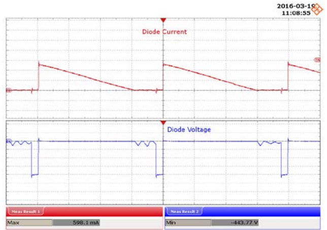
Figure 62 – 265 VAC, 385 V LED Load. Upper: I_{D1} , 200 mA / div. Lower: V_{D1} , 100 V / div., 5 μs / div.
