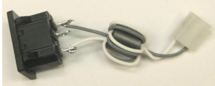
Figure 43 – Supplemental CM Choke (4T on Fair-Rite 5943000201).
