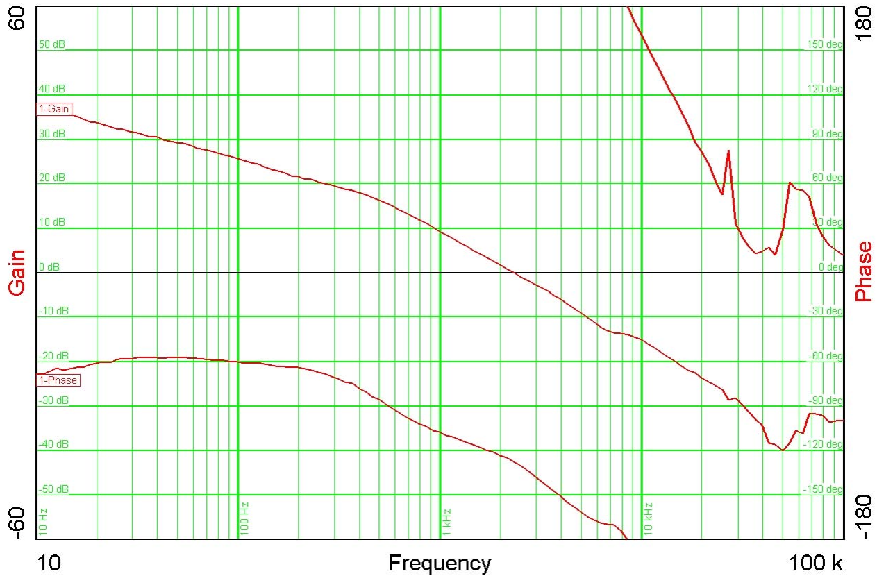
Figure 35 – Gain-Phase Plot, Maximum Steady-State Load. Vertical Scale: Gain = 10 dB / div., Phase = 30 ° / div. 110 VDC – Crossover Frequency = 2.3 kHz Phase Margin = 50°.
