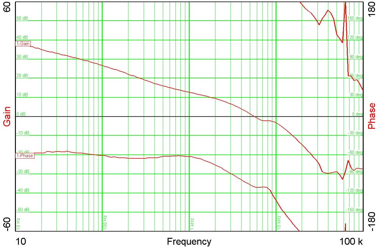
Figure 36 – Gain-Phase Plot, Maximum Steady-State Load. Vertical Scale: Gain = 10 dB / div., Phase = 30 ° / div. 380 VDC - Crossover Frequency = 5.5 kHz Phase Margin = 70°.
