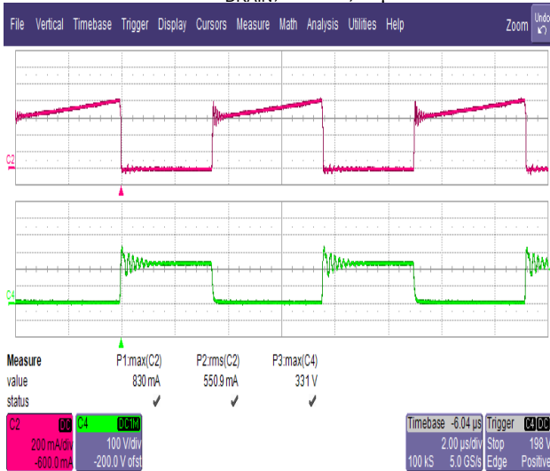
Figure 21 – 110 VDC, Over Load (125%). Upper: I_{DRAIN} , 0.2 A / div. Lower: V_{DRAIN} , 100 V, 2 \mu s / div.
