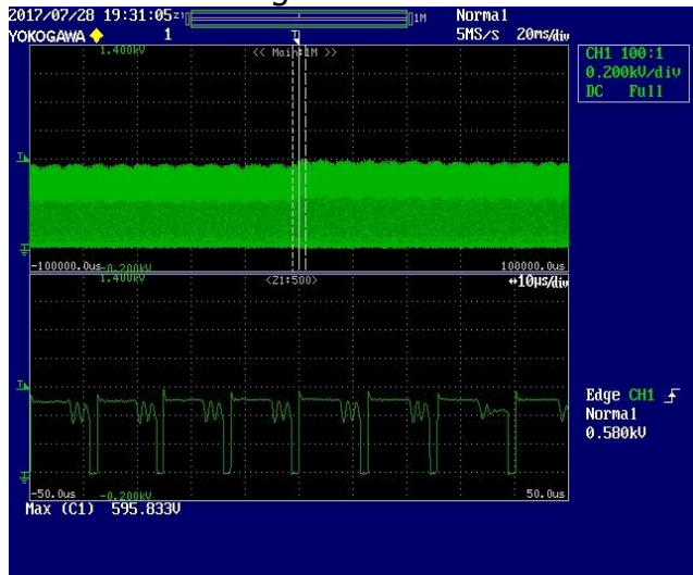
Figure 123 – (+)1 kV Differential Surge. 90° Phase Angle, Input: 277 VAC. V_{DRAIN} , 200 V / div., 20 ms / div. Peak V_{DRAIN} : 595.833 V.
