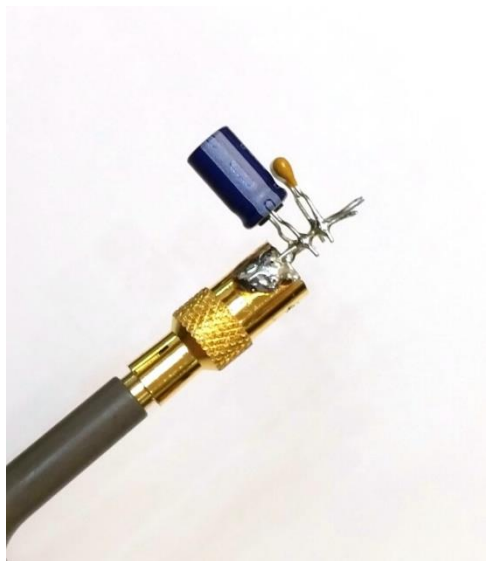
Figure 105 – Probe Set-up for Output Voltage Ripple Test.
