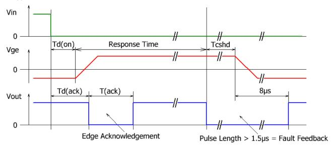
Fig. 9 Driver behavior and status feedback in the IGBT short-circuit condition
