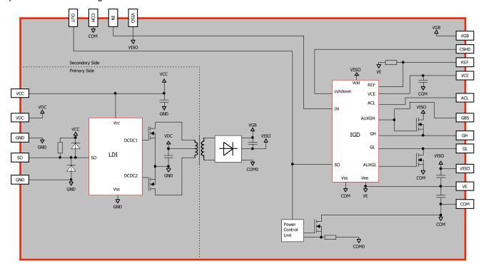
Fig. 2 Block diagram of the 1SC0450E2A0 driver core
