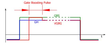
Fig. 12 Gate-boosting signals
