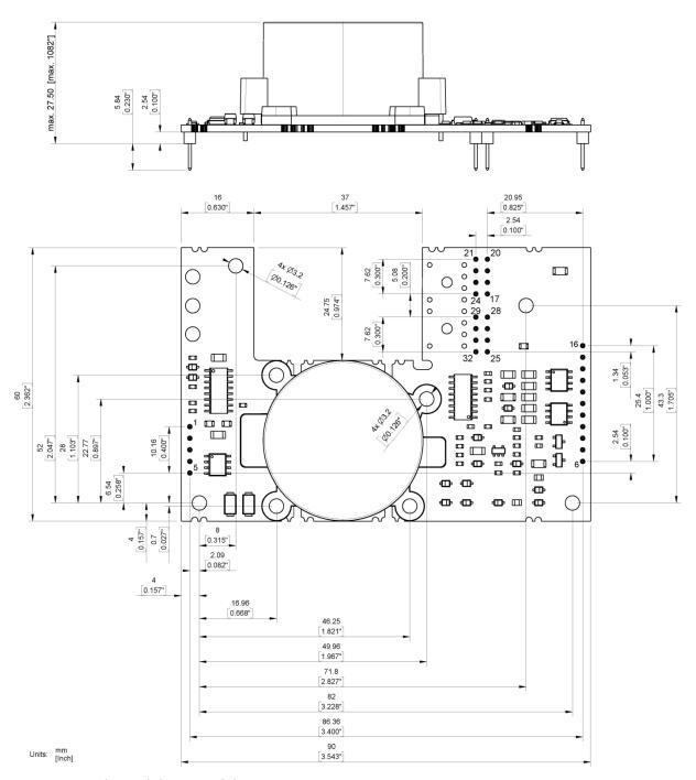
Fig. 4 Mechanical drawing of the 1SC0450E2A0
