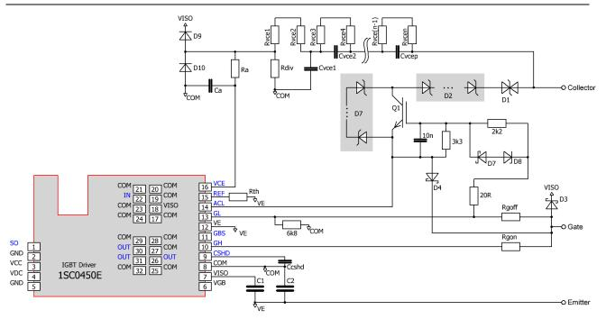
Fig. 6 Recommended user interface of the 1SC0450E2A0 (secondary-side pins 6 to 16) without gate boosting (refer to chapter "Gate Boosting" and Fig. 11 for gate-boosting circuitry)
