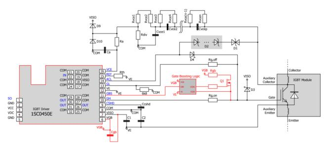
Fig. 11 Gate-boosting circuit principle – highlighted in red color
