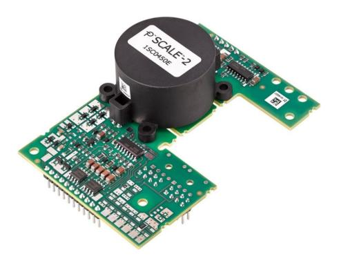
Fig. 1 1SC0450E2A0 driver core
