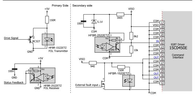
Fig. 7 Recommended command interface circuitry with Avago fiber-optic links HFBR-x522ETZ
